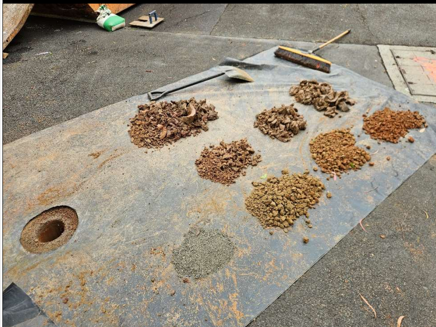
PHOTO 24: BH104 (NORTH OF SITE) SOIL PROFILES EXTRACTED BY SOLID FLIGHT AUGER
