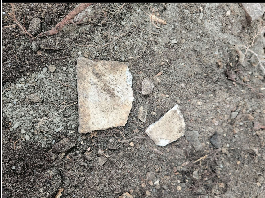
PHOTO 16: ASBESTOS FRAGMENTS OBSERVED AT TP105 (NORTH-WEST OF SITE) AT 0.1 – 0.6 M BGS
