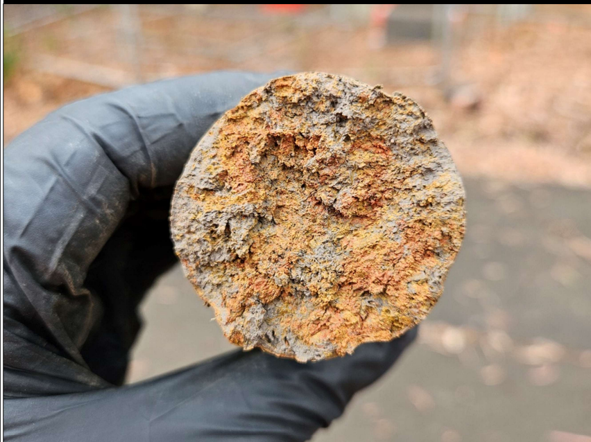
PHOTO 24: BH104 (NORTH OF SITE) SOIL PROFILES EXTRACTED BY SOLID FLIGHT AUGER
